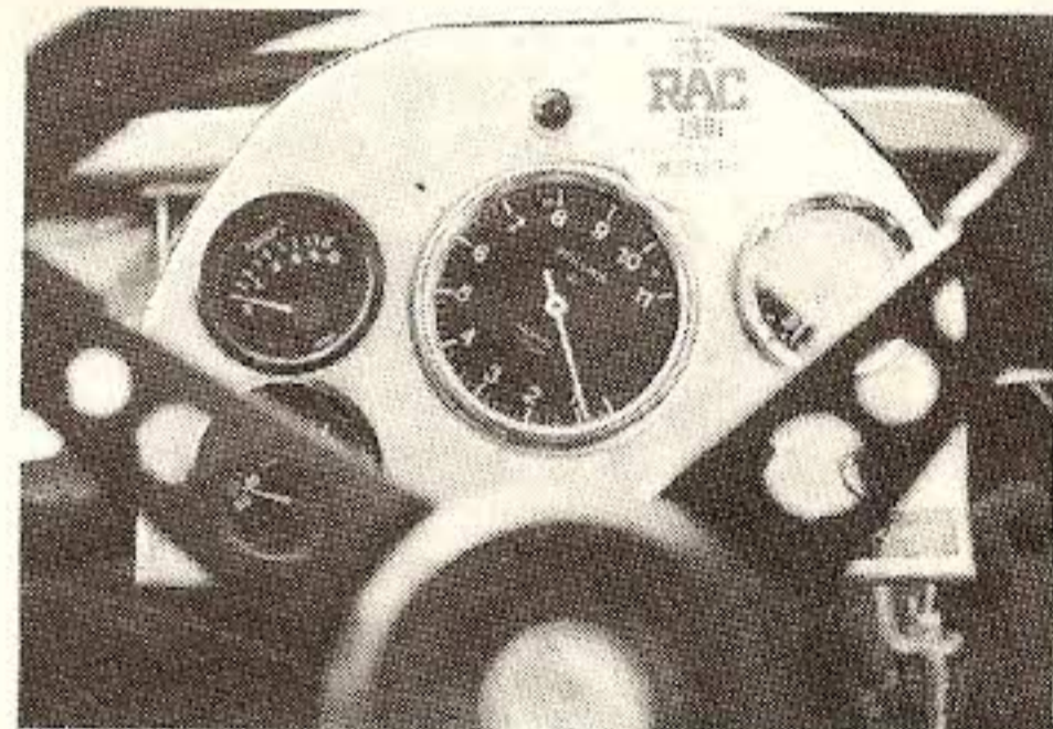
THE basic instrument panel, showing the Race Parts tachometer which was replaced between Goodwood and Brands Hatch due to lack of a suitable drive.
